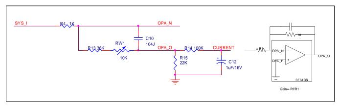
Figure 2-6 Current Measurement Circuit
